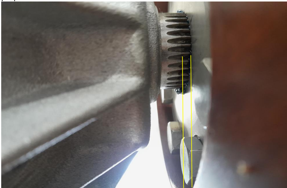
Photo 2. Measurement points between the yellow lines. Must be 2mm or greater.
